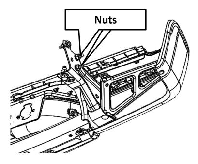
Install the bumper step onto the studs. Then reinstall the factory nuts that were removed in step one. <u>Fully tighten the hardware.</u>
